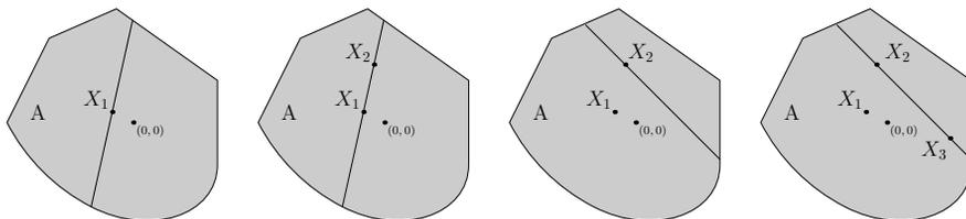
Fig. 1. Illustration of the generation of  $X_3$  and  $X_2$  by the hit-and-run algorithm given state  $X_1$
