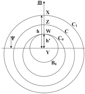
Fig. 1. Heights along the common normal  $\mathbf{m}$
