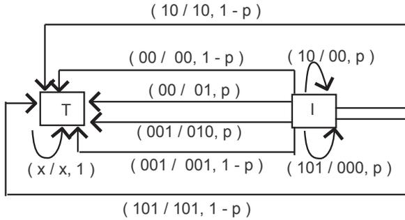
Fig. 2. Transducer of the Fibonacci fallible adding machine
